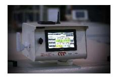
Our TCX 4.0 Touch screen control offers you the possibility to have all standard functions and programmable momories, all System can be connected to LAN.
