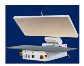
This little magnetic tensfer / fusing machine allow to fuse jacket Parts and sportwears, it allow also to make transfer and sublimation. This machine doesn't need air comprimed.
