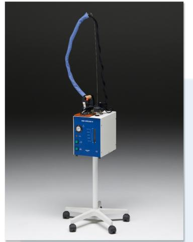
industrial steam generator with round boiler 5 Liters, pressure switch for exact control of steam pressure, visual control of the waterline in the boiler, ball valve for deposit and water outlet, steam valve with control of steam flow, safety valve cap, No. 02 safety thermostats to protect the heating elements in case of lack of water and to protect the boiler against too high temperatures.
