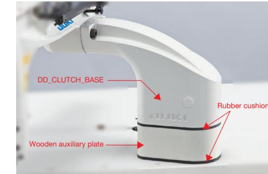
The MT-05 (DD\_CLUTCH\_BASE asm) is required to install the belt-drive type sewing machine on the table.
